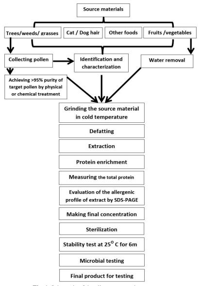
**Fig. 1.** Schematic of the allergen extraction process.
