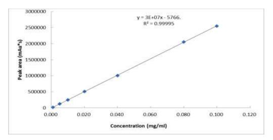
**Fig. 2.** The calibration curve of Orcinol -  $\beta$  - D - glucoside in HPLC fingerprinting: The signal E+7 means  $10^7$ .
