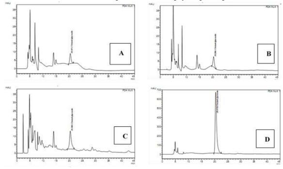
**Fig. 3.** HPLC chromatogram of the dry rhizome of *Curculigo orchioides* Gaertn. extract visualized by A) CT-3, B) CT-2, C) CT-1, and D) CT-4. The vertical axis is intensity (mAU), the horizontal axis is retention time (min). The retention time of Orcinol-β-D-glucoside compound in 4 formulas are all around the 20th minute.
